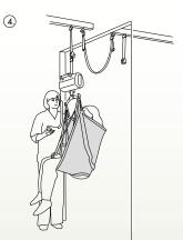
When the patient has been transferred to room 2 completely, the Strap Gripper is removed from the Room-to-Room Strap and the transfer along the rail can continue.
