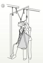
When the patient's weight is completely transferred to the Room-to-Room Strap, the lift strap is removed from the Quick-Release Hook in room 1.
