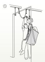
Attach the Strap Gripper to the Room-to-Room Strap and lower the lift. The patient's weight is gradually transferred to the Room-to-Room Strap.
