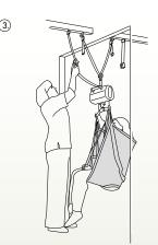
Then attach the lift strap to the Quick-Release Hook in room 2 and run in the lift strap. The patient is now transferred to room 2.
